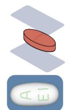
Two 3D laser sensors (a must have) ensure tablet surface analysis covering cracks, embossment, thickness defects, coating and engraving integrity
